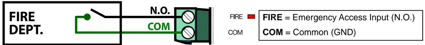
The fire input is meant to allow emergency personnel the ability to open the gate in an emergency situation without needing assistance. See the following section, "Emergency Gate Access", for more information.
